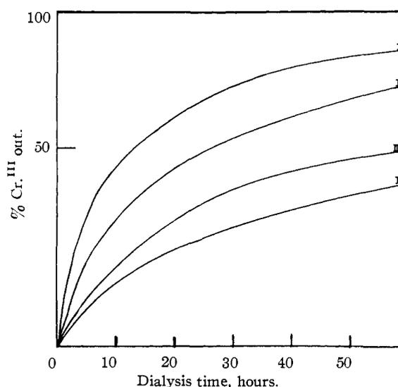
Fig. 4.—Rate of diffusion of chromic acetate in  $\mu = 0.1$ , acetate and phosphate buffers at 5-8° as a function of pH: I, pH 4.14; II, pH 5.30; III, pH 6.40; IV, pH 7.35.
