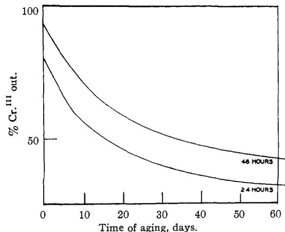
Fig. 3.—Diffusibility of  $8.40 \times 10^{-3} M$  chromic acetate in  $\mu = 0.1$ , phosphate buffer at  $5-8^\circ$  ( $pH$  7.35).
