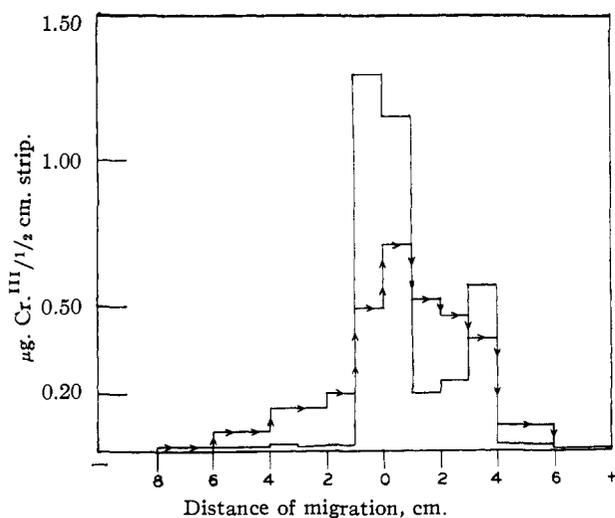
Fig. 2.—Paper electrophoresis of chromic acetate in  $\mu = 0.1$ , phosphate buffer  $pH$  7.35: I (---),  $6.44 \times 10^{-3} M$  by dilution of 27-day old  $0.655 M$  solution; II, (—),  $6.44 \times 10^{-3} M$ , 27 days old.
