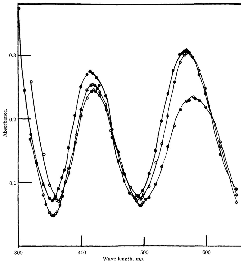
Fig. 5.—Absorption spectra of  $8.19 \times 10^{-3} M$  chromic acetate at various  $pH$ 's: (I)  $\circ$ ,  $pH$  4.86; (II)  $\bullet$ ,  $pH$  6.30; (III)  $\ominus$ ,  $pH$  11.20.
